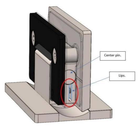
Normally when loosening the small screws, these lip areas lose their grip and hold. But sometimes the areas keep the hold. This means the indicated area (on both sides of the hinge) needs to be spread apart for the centrer pin to rotate freely.
