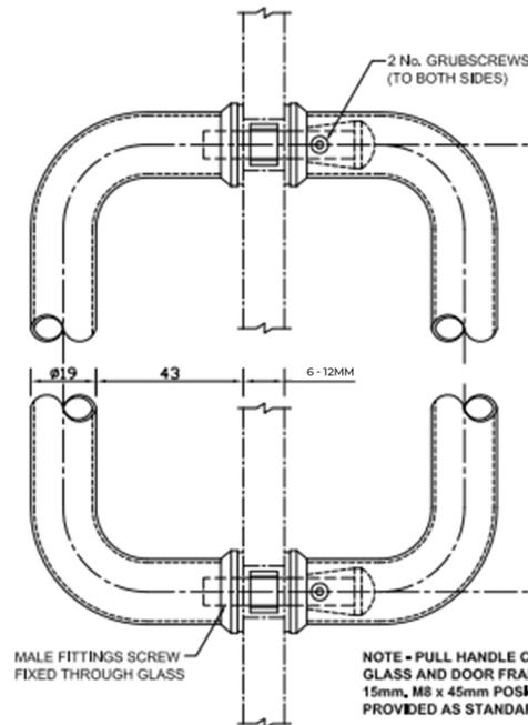
**NOTE - PULL HANDLE CAN BE UTILISED ON GLASS AND DOOR FRAMES THICKER THAN 15mm, M8 x 45mm POST-PAN SCREW PROVIDED AS STANDARD FOR 15mm MAX.**
