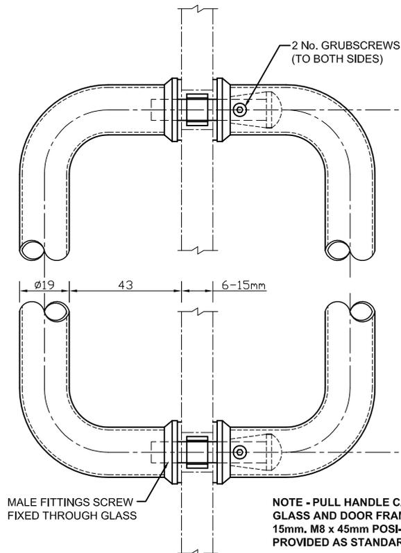
NOTE - PULL HANDLE CAN BE UTILISED ON GLASS AND DOOR FRAMES THICKER THAN 15mm. M8 x 45mm POSI-PAN SCREW PROVIDED AS STANDARD FOR 15mm MAX.
